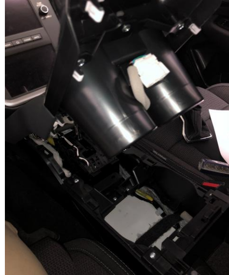
Lift towards rearward to remove console cover and place upside down on protected bench top
