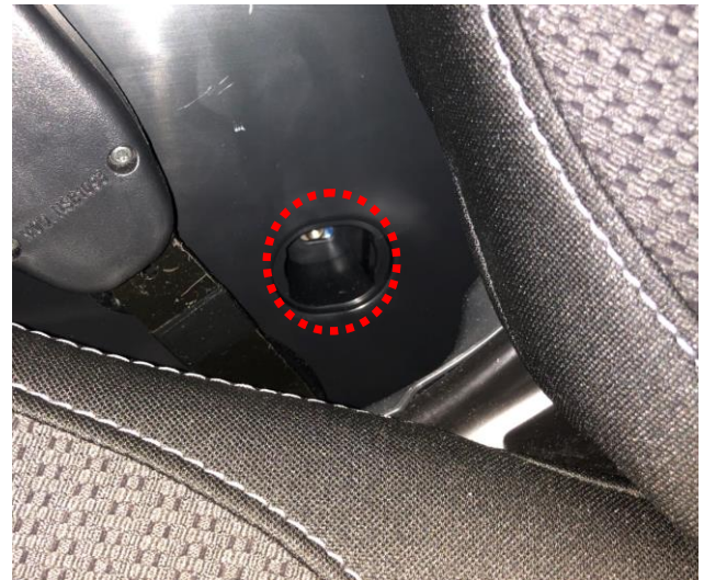
On the driver side of the console box, remove round trim insert and remove 10mm bolt.
