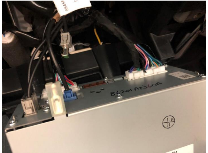
Disconnect all remaining connectors from radio and carefully place unit aside.
